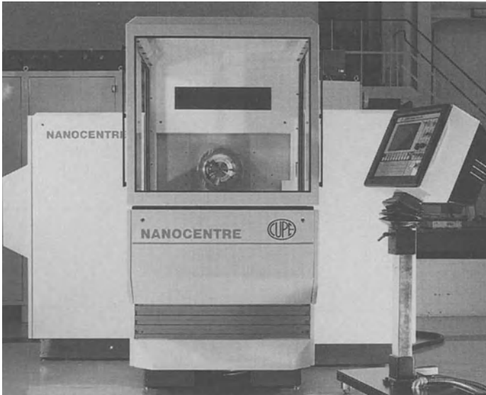
Fig. 2.27. Possibly the most accurate and advanced diamond turning/grinding centre at present available. [Courtesy of CUPE Ltd.]
