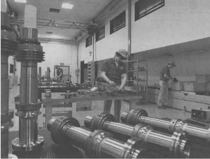
Fig. 2.23. The clean room and sub-assembly area for critical parts, such as spindles and headstocks (turning centres), also spindle cartridges (machining centres) prior to complete machine tool assembly. [Courtesy of Yamazaki Mazak Ltd.]
