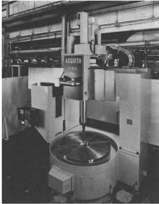
Fig. 1.49. A CNC vertical turning lathe. [Courtesy of Asquith 81.]
