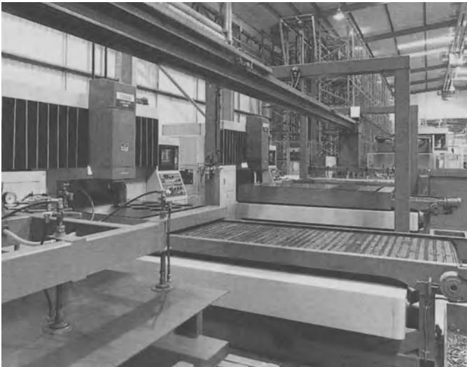
Fig. 2.20. Sheet metal working – laser path cutting machines, CNC folding and bending machines, together with automatic welding machines. [Courtesy of Yamazaki Mazak Ltd.]
